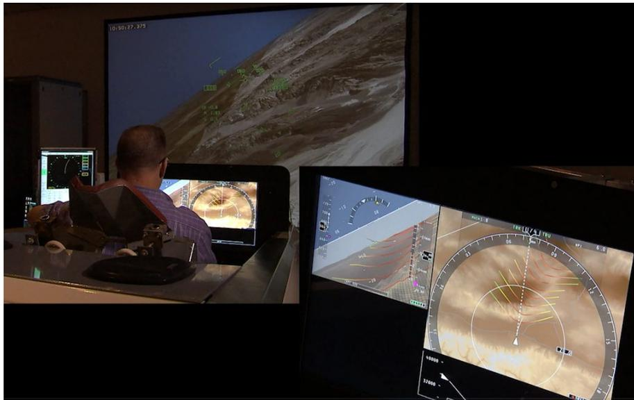
Figure 8: Sonic boom display integrated into NASA's QueSST simulator at NASA Armstrong Flight Research Center.
