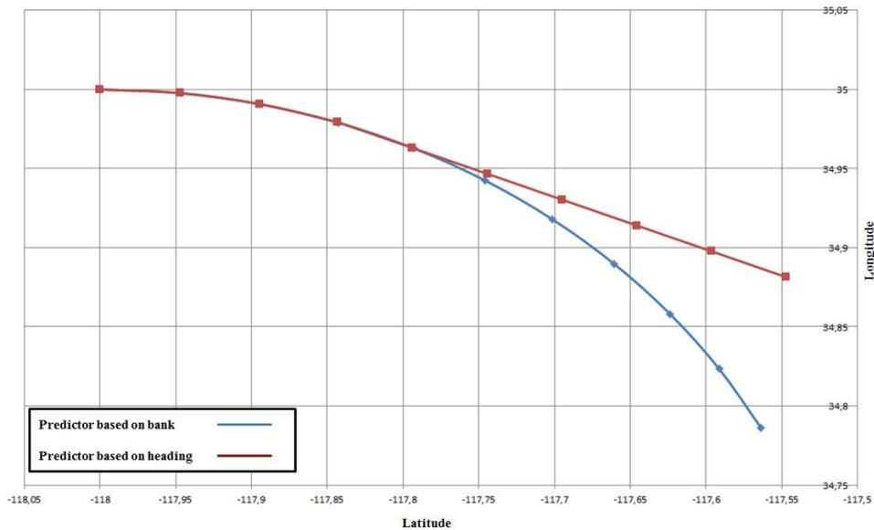
Figure 4: Differences in predicted trajectory using bank angle (second order predictor) & heading (first order predictor).
