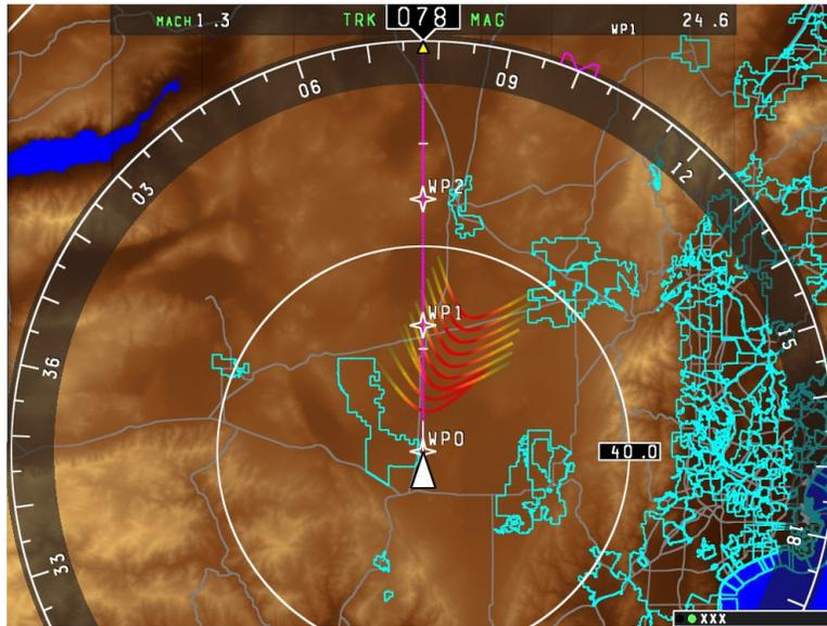
Figure 6: Sonic Boom Footprint via first order predictor that uses heading for trajectory prediction. A first order predictor using heading assumes an instantaneous rate of turn to go from current heading to selected heading. This introduces error into the prediction for larger heading changes.
