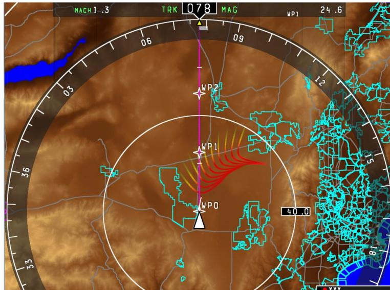
Figure 5: Sonic Boom footprint via second order trajectory prediction that uses bank angle for trajectory predictions. The second order predictor is used for the period of time that the aircraft is expected to be turning (using standard rate turns to selected heading).
