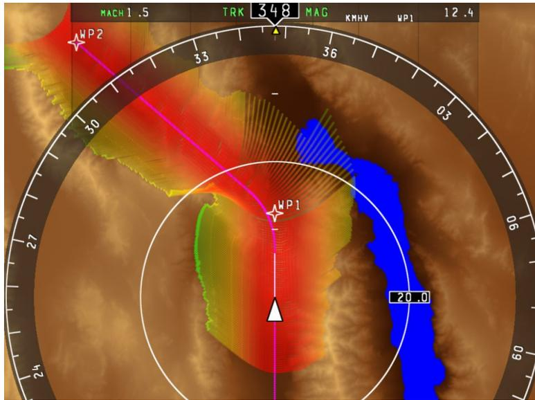
Figure 2: Sonic Boom Display prototype illustrating mountain occlusion of the boom carpet.
